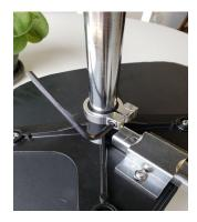
Using the smallest Allen wrench, back out the set screw by rotating to the left
