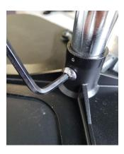
Remove the old seat post and insert the bushing, lining up the slot on the bushing with the slot on the seat plate
