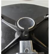
Insert the seat clamp, install the suspension seat, and tighten the seat clamp
