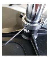
Use the same Allen wrench to remove the large seat post screw
